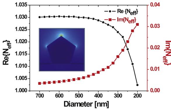
**Figure 5.** Calculated dispersion of the real and imaginary parts of the surface plasmon effective index as a function of the nanowire section. The inset shows a cross-sectional intensity distribution of the leaky plasmon mode for a pentagonal Ag nanowire with a section of 300 nm.
