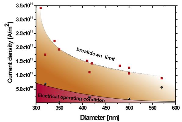
**Figure 6.** Current densities leading to electrical failure of crystalline Ag nanowires (squares) and degradation of surface plasmon characteristics (circles) as a function of nanowire width, respectively. The pink shaded area qualitatively indicates the safe electrical operating condition to simultaneously propagate electrons and surface plasmons in the metal nanowires.
